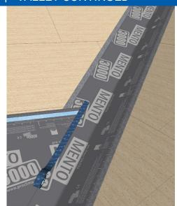
Beginning on the bottom of one side of the valley, overlap a sheet of MENTO 3000/5000 over the gutter, extending approximately halfway into the field. Seal the membrane edge with TESCON VANA tape.
