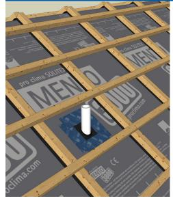
Airseal pipes with ROFLEX air sealing sleeves. ROFLEX 20 is self-adhering with integrated TESCON VANA patches. Other ROFLEX pipe sleeves should be adhered to MENTO with TESCON VANA.
