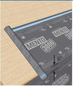
Unroll membrane perpendicular to pitch along the entire length of the roof section with the writing on MENTO 3000/5000 facing outward.
