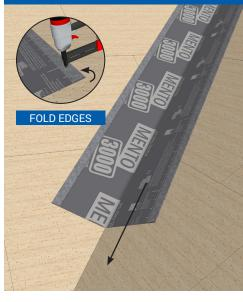
Install a MENTO gutter by laying a partial sheet of MENTO 3000/5000 from top to bottom of the valley. Fold the edges of the membrane about 3" and secure sparingly, creating a back-dam.
