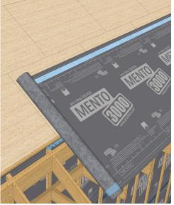
Align bottom membrane edge with eave and unroll sheet perpendicular to pitch along the entire length of the roof section. The writing on MENTO 3000/5000 should face outward. Secure to the wall membrane with TESCON PROFIL tape.
