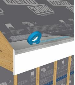
Membranes to extend over a gutter or drip edge flashing shall be fixed without creases with DUPLEX or TESCON VANA tape so water will drain away and the membrane is permanently secured.
