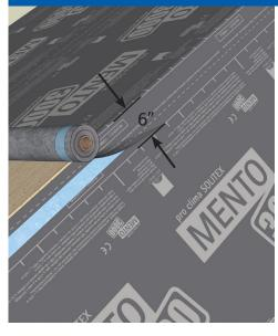
Extend one sheet of MENTO over the ridge and overlap this edge of membrane over the MENTO on the other side by at least 6".
