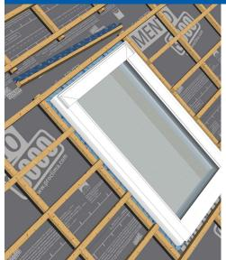
A subroof gutter above a roof obstruction such as a skylight or chimney should be made with a pitched batten. Attach batten to MENTO using TESCON VANA. This batten will direct all rainwater to a roof area without obstructions.
