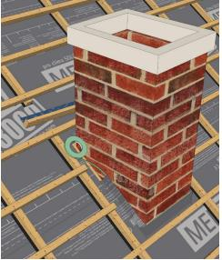
Create a subroof gutter for transverse drainage above the chimney using a pitched batten attached to the MENTO using TESCON VANA. Secure MENTO to the chimney using CONTEGA MULTIBOND or CONTEGA HF.
