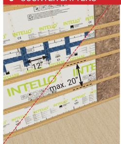
Add horizontal counter battens spaced max. 20" apart before dense packed insulation is blown in. Tape joint should be supported with a batten over the tape or reinforced with perpendicular strips of tape spaced less than 12" apart.
