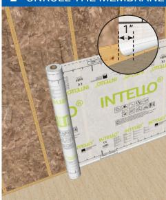
Unroll INTELLO for the entire wall section, allowing sufficient material for "relaxed" corners at intersecting wall studs. Ensure there is a 1" overlap of the membrane covering the floor for future sealing (in step 7).
