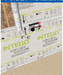
Using the printed markings as a guide, overlap the next row of INTELLO over the bottom sheet and staple along the bottom edge. As in Step 3 - pull the membrane up into a taut triangle and fasten at the upper edge.
