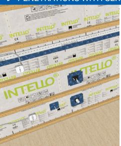
Airseal pipes and cables with ROFLEX and KAFLEX air sealing sleeves. The cable sleeves and ROFLEX 20 are self-adhering with integrated TES-CON VANA patches. Other ROFLEX pipe sleeves are adhered to INTELLO with TESCON VANA.
