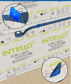
Use TESCON VANA to tape the INTELLO overlaps. Use the dotted line to center the tape over the joint and press firmly with a PRESSFIX tool. The higher the initial pressurization, the more secure the bond will be.
