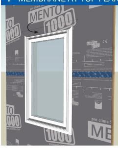
Unfold the membrane and run it over the top flange.
