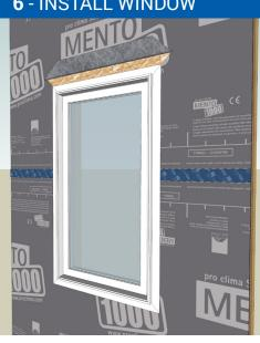
Install the flanged window and fasten to structure per manufacturer's instructions.
