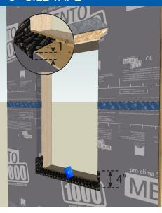
Install EXTOSEAL ENCORS on window sill, extending it up each side a minimum of 4". Use PRESSFIX to accurately press into
