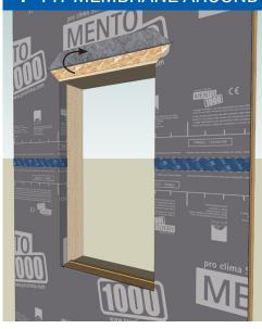
Fold up upper part of membrane and temporarily hold in place with masking tape. This is so it can be installed over the header flange of the window later.
