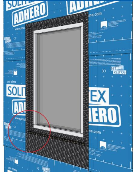
Seal frames with CONTEGA SOLIDO EXO to taped window bucks. Start on the bottom and work your way up for proper shiplapping. Use pre-made L-shaped corners for most accurate sealing of corners. Apply tapes to windows as per manufacturers recommendations and installation instructions-note drainage planes, condensation weeps etc. Pressurize tape firmly with a PRESSFIX.
