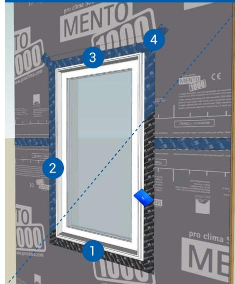
(1) Use 2 3/8" TESCON VANA or CONTEGA SOLIDO EXO tape to seal the bottom flange to the membrane. Press firmly with a PRESSFIX tool (typ.)
