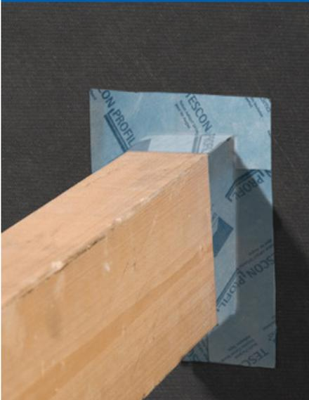
Waterproof and air sealed connections to beams, can be made with TESCOIN PROFIL tape. Cut the tape 2" (50 mm) longer than the beam dimensions.
