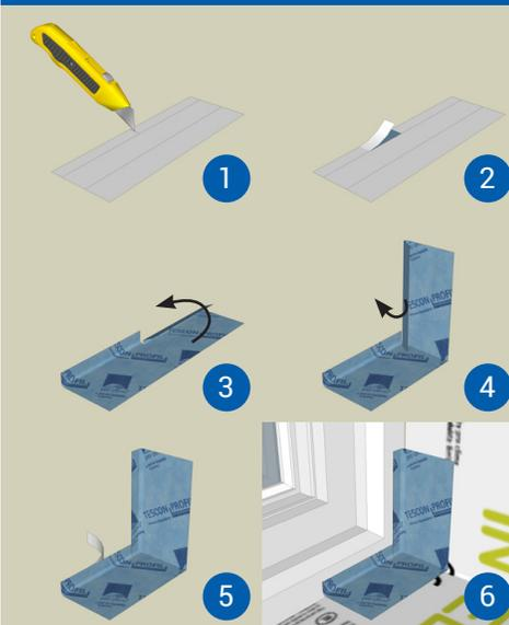
(1) On a 4-6" long piece of TESCON PROFIL/PROFECT/SOLIDO SL tape, cut through the narrow section of the tape - stay 1/16" from edge. Pre-fold tape at cut location.
