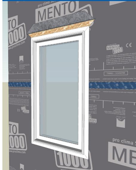
Install the flanged window and fasten to structure per manufacturer's instructions.
